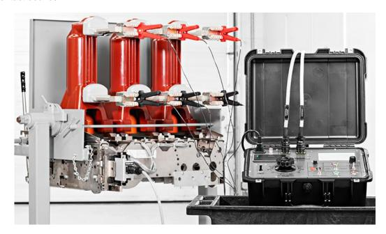
With the integrated variable 120 VAC/125 VDC power supply, the CBT-1203 can operate breakers outside of cubicles. Breaker switching controls and custom breaker-specific operation plugs allow users to quickly set up and operate the unit with all types of circuit breakers. The large back-lit LCD display is viewable in sunlight and low-light conditions.
