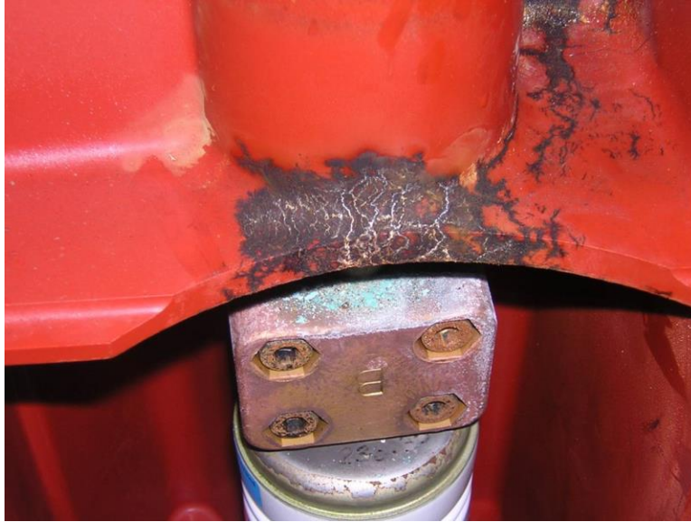
Effects of Unmitigated Partial Discharge in Insulation Figure 11
