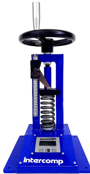
Wipe Spring Spring Rate Test Setup Figure 8
